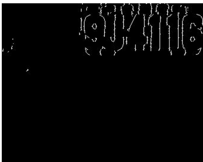
Fig. 8: The results of the edge detection by Sobel vertical filter
